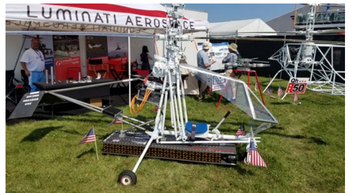
In Oshkosh, Wisconsin, in July, Luminati had fitted the battery pack and electric motor to the Rotorcycle. Dr. Zucker explains the Polarix motor in the background next to a frame for the larger QH-50 rotor system. (VFS staff photo)
