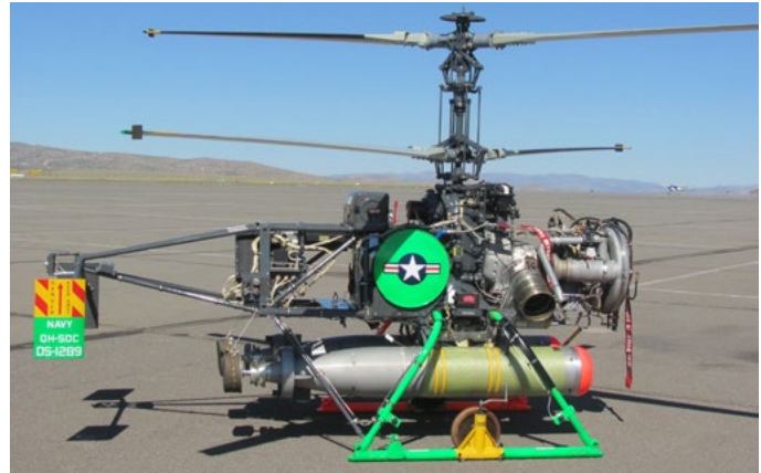
The unmanned QH-50 Drone Anti-Submarine Helicopter (DASH) was developed in the 1950s to find and kill enemy submarines. (Luminati photo)
