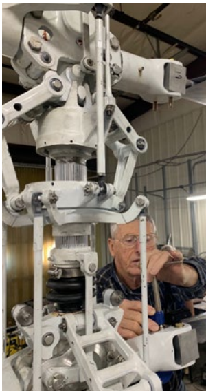
Dick Degraw adjusts the Rotorcycle rotor head assembly (Luminati photo)
